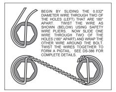
Figure 3. Safety Wire Diagram
