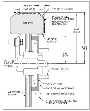
Figure 2. Wheel Clearance Diagram
